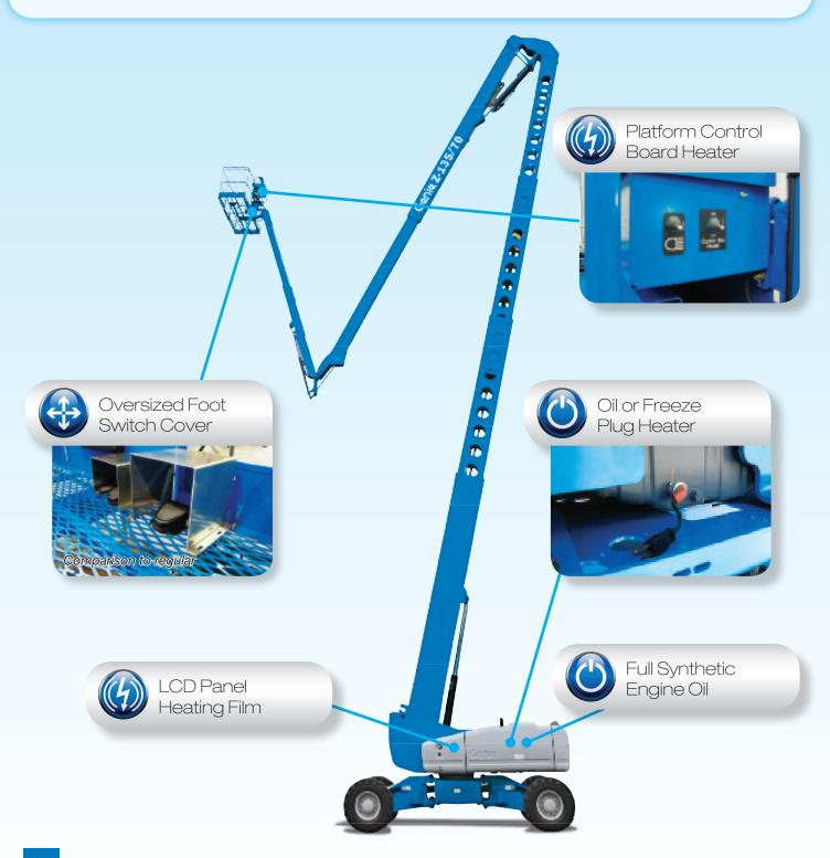
Package contents vary to accommodate various boom model configurations, and protect different areas of the machine's operation:
